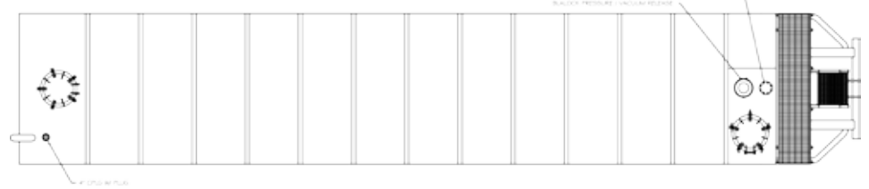
Dimensions Pictured: 45' long, 8'-6" wide, 10' high; 500 barrel capacity
